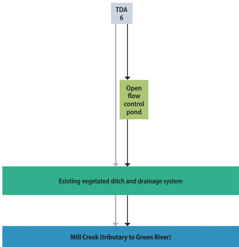
Not to scale. Diagram depicts flow paths only. Size of text boxes and length of arrows do not represent actual area of, or distance between, drainage features.
