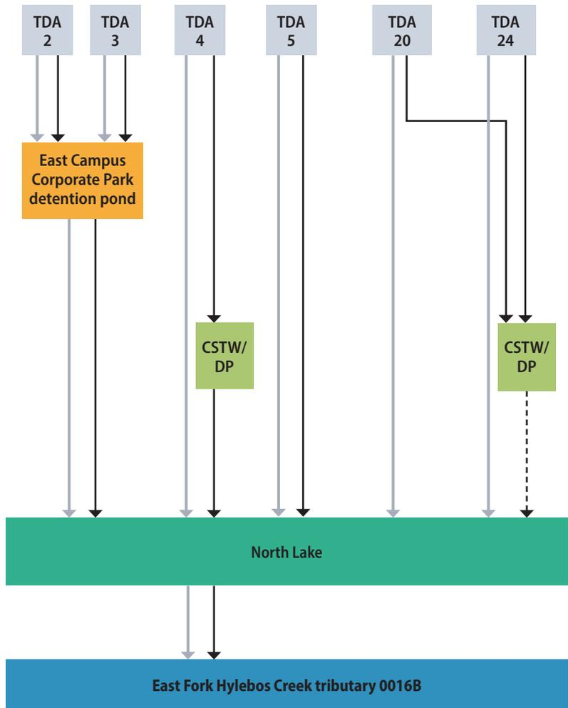
Not to scale. Diagram depicts flow paths only. Size of text boxes and length of arrows do not represent actual area of, or distance between, drainage features.
