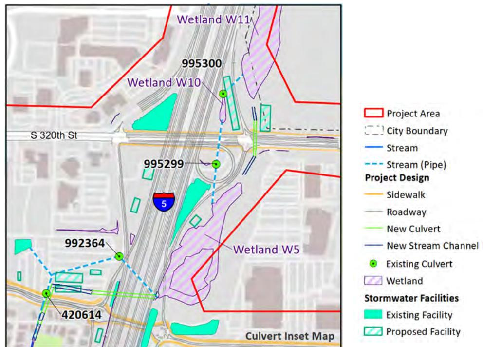
**Figure 2.** Existing Culverts to be Replaced
