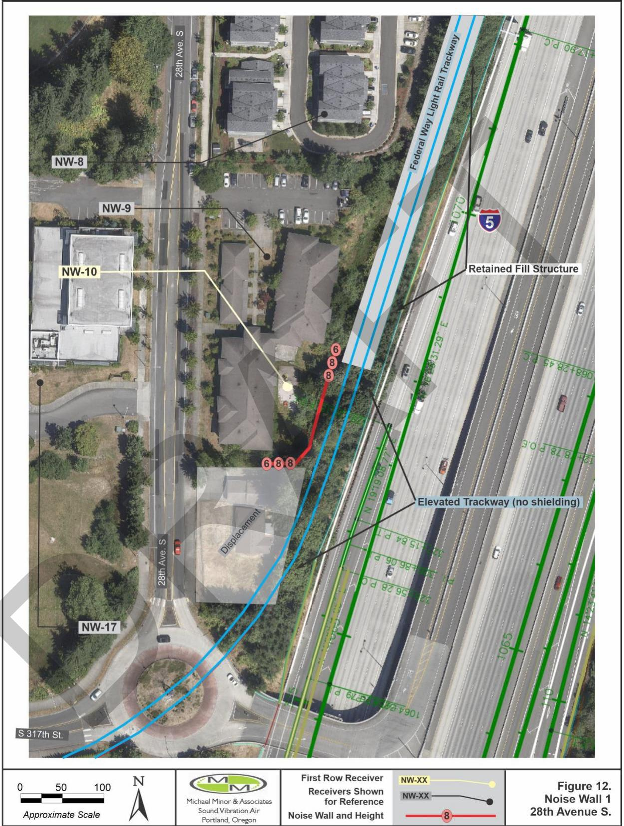
Noise Wall 1 has a total length of approximately 185 feet and is designed to provide noise abatement for the first row residences represented by receiver NW-10. The heights of the panels range from 6 to 8 feet, with a total area of 1,446 square feet (SF). Using the standard cost from WSDOT of \$51.61 per square foot, the cost of the wall is \$74,628.
