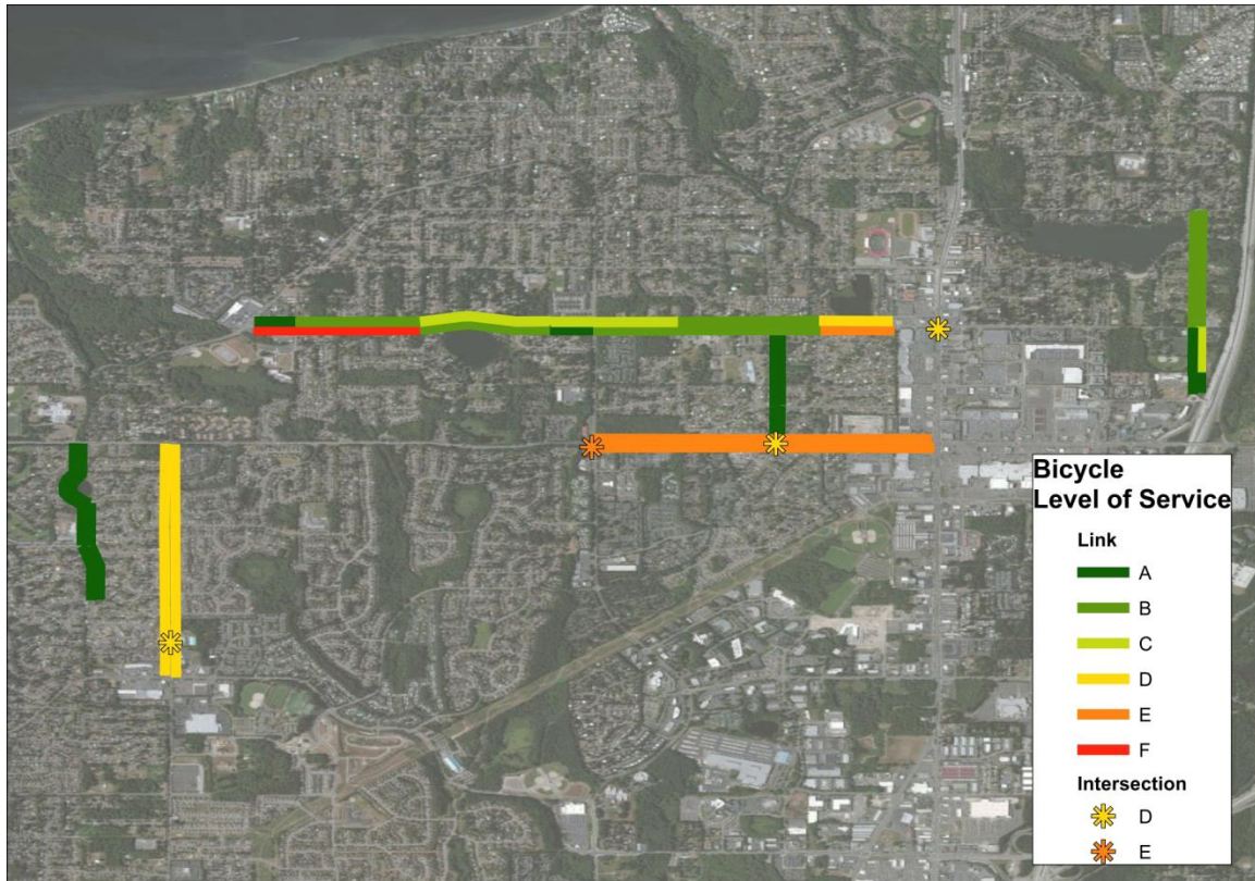
Figure 3.X – Bicycle Level of Service for Representative Corridors
