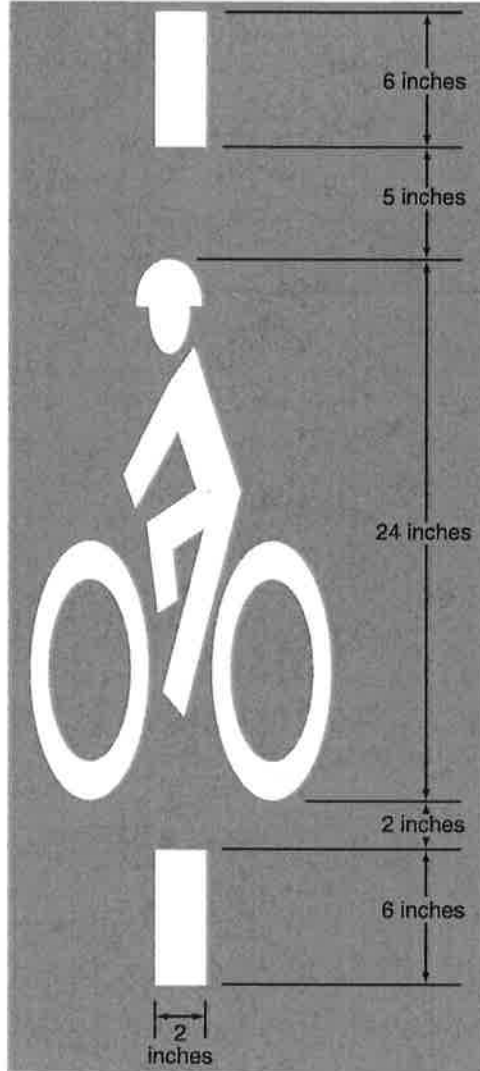
Figure 9C-7. Bicycle Detector Pavement Marking
